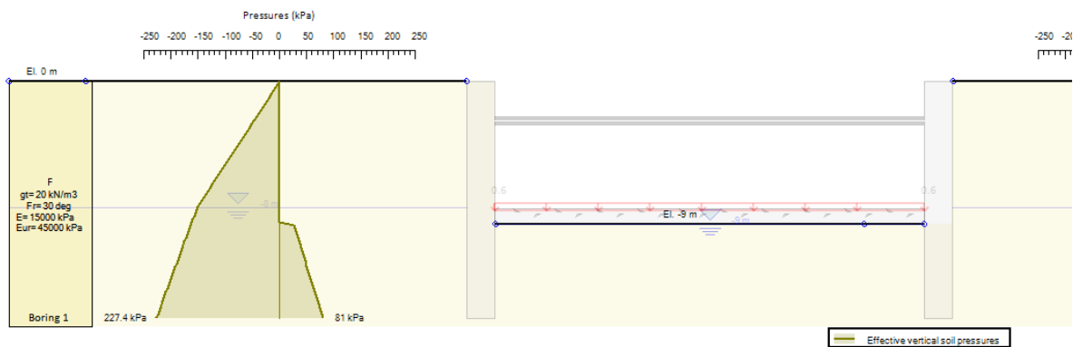
Stage 4: Vertical effective stresses with slab included (no lining effect). Note: 55.4 kPa + Slab dead 25 Kpa + Slab live load 0.6 kPa = 81 kPa
