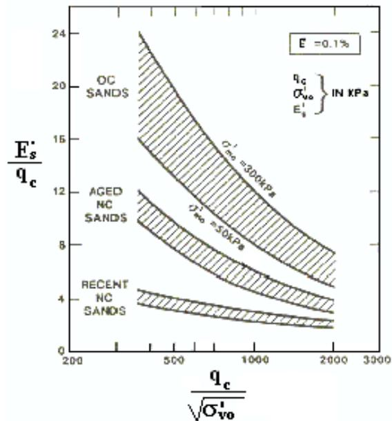
Figure 8: Estimation of secant modulus of elasticity for sands from cone penetration tests (Brinkergreve, 2002)
