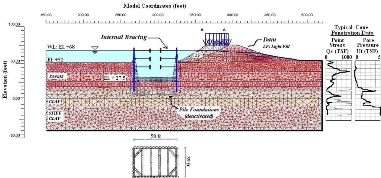
Figure 11: Finite element model at final subgrade
