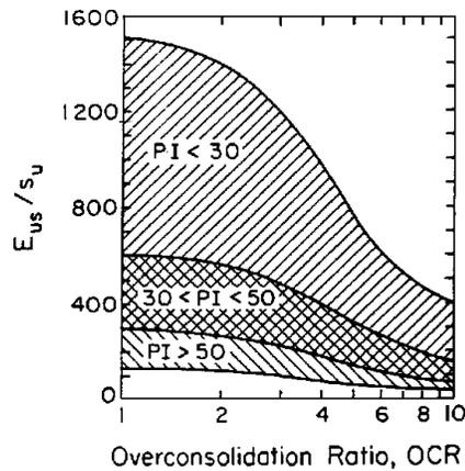
**Figure 9: Generalized Undrained Modulus Ratio versus OCR and PI**
