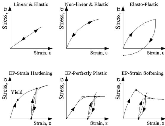
**Figure 3: Idealized Modes of Elastic Soil Behavior (Whittle, 2005)**
